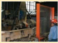
Koppers also has two framing mills where specialized track and bridge components are made.
